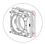
Align rubber seal and mounting flange-seal packing and insert screws with washers in wall plugs.
