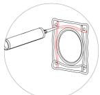
For additional sealing and adhesion, apply UGA-Sikaflex-11 FC (not included in the scope of supply) in a grid pattern around the holes, in the area of the mounting surface.
