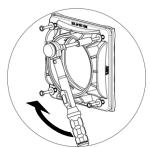
Screw in the screws (width across flats 13 mm) up to the stop. The wall plug is correctly anchored if, once the screw has been screwed in fully, the wall plug does not rotate and it is not possible to turn the screw any further.
