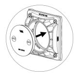
If immediate mounting of a system cover is not intended, the protective cover/PE cover must be pressed back into the mounting flange as protection.
