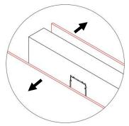
Remove the casing after the concrete has hardened.
