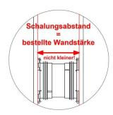
The casing spacing must not be less than the specified wall thickness of the entries ordered.
