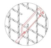
Cut out the rebar reinforcements around the wall insert.
