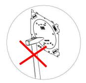
Do not open with force to avoid damage to the bayonet mount and the sealing surfaces.
