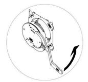
Unscrew the system cover counter-clockwise using the UGA articulated spanner "GSS".
