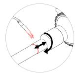
After the shrinking area on the cable/pipe has cooled, continue until the thermal sleeve is crease-free and completely encompasses the cable/pipe, so that the hot-melt adhesive emerges evenly out of the thermal sleeve all round.
