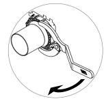
Tighten the union nut with the UGA articulated face wrench "GSS" until the system cover cannot be turned any further, and it is no longer possible to lightly turn the union nut.
