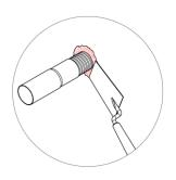
• Mortar the flexible house infeed in the hole, so that the red lining sits approx. 1 centimetre inside the hole area.
