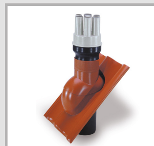
MSD110 with seven connection pieces and six thermal shrink sleeves One connection piece is supplied closed and can be opened if necessary; Suitable for max. four cables with a diameter of 7-23 mm and max. three cables with a diameter of 7-30 mm; Various AK spreader caps or VS25 sealing plugs are available as accessories
