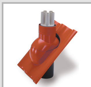
MSD110 with five connection pieces and five thermal shrink sleeves Suitable for five cables with diameter 7 – 18 mm; Various AK spreader caps or VS20 sealing plugs are available as accessories
