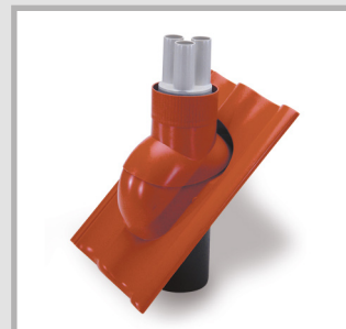
MSD110 with three connection pieces and three thermal shrink sleeves Suitable for three cables with diameter 7 – 28 mm; Various AK spreader caps or VS30 sealing plugs are available as accessories.
