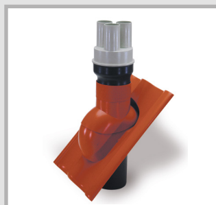
MSD110 with three connection pieces and three thermal shrink sleeves Suitable for three cables with diameter 16 – 44 mm; Various AK spreader caps or VS46 sealing plugs are available as accessories.
